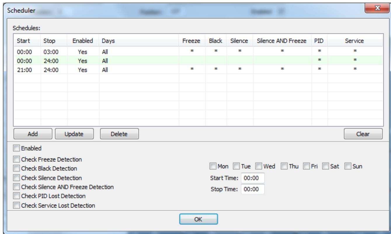
If a test is not used in the 'Configure Wall' setup, it will be shown grey in the Schedules overview list.
