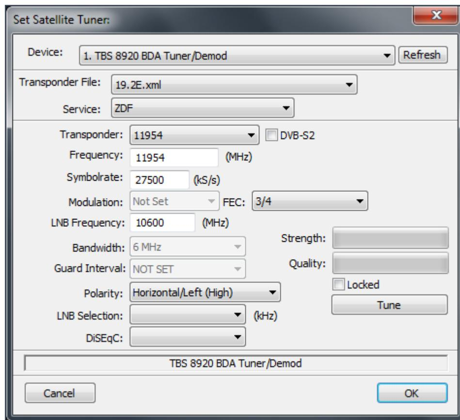
When multiple BDA driver adapters are installed, they can be selected via de Device pull-down menu.
