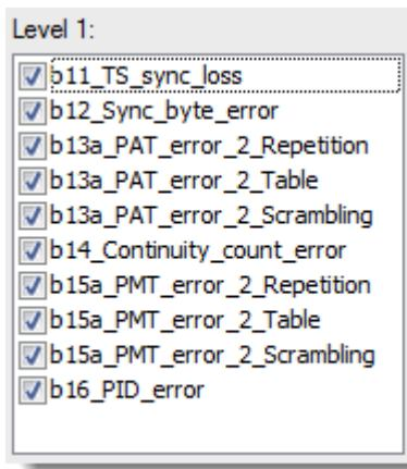
If enabled, ETR290 level 1 faulty situations are signalled.
