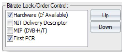
Selection in which priority (via Up/Down) the Transport stream bitrates method is used:
