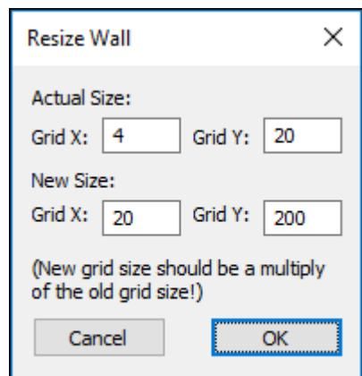
In the ‘Resize Wall’ the new Grid X and Y size can be given. Of course the new size has to be a multiple of the original size.
