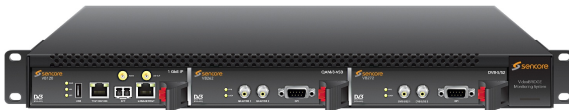
Figure 4.1: The Enhanced Chassis with probe boards installed
