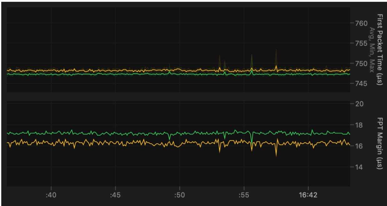
The second two graphs show *First Packet Time* and *FPT Margin*. The *First Packet Time* graph shows the time difference between the packet's timestamp at arrival and the Alignment Point. While the *FPT Margin* graph shows the time difference between the packet's timestamp at arrival and start of packet read.
