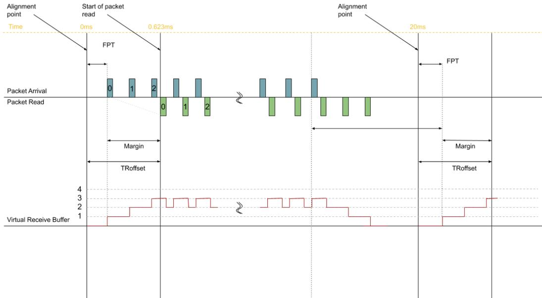
The figure above illustrates the timing model, which puts constraints on the timing of packets on the output of the sending device. The network compatibility model (C), Virtual receiver buffer (VRX) and packet read schedule (PRS) all ensure that the delivery timing is overhauled by shaping the transmission.
