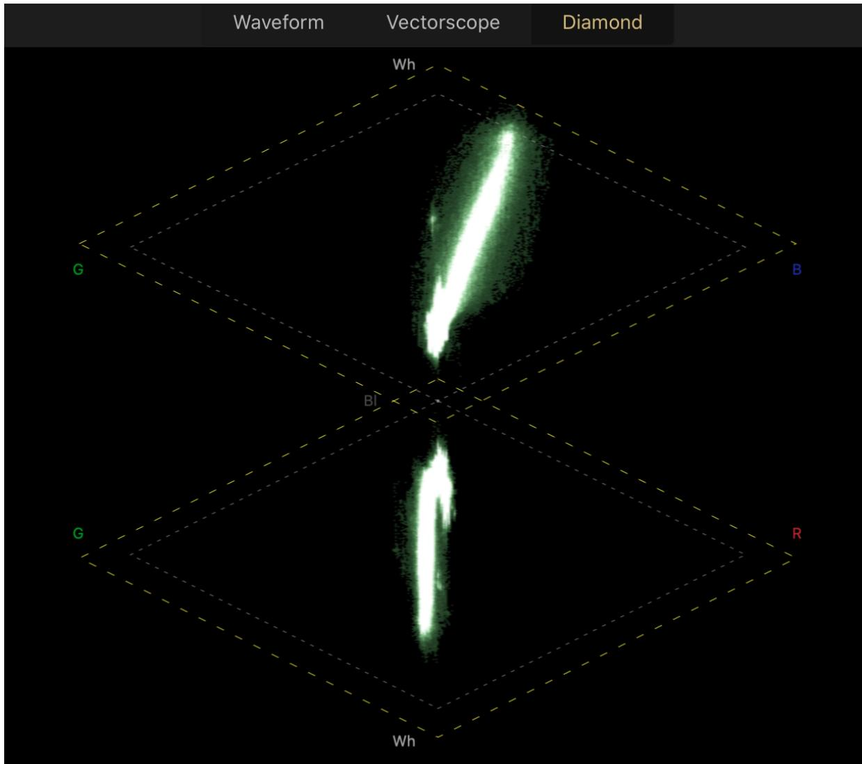
The Diamond scope shows the interaction of RGB and helps identify RGB gamut errors in digital video signals. The blacks are in the middle of the display where the two diamonds join. The whites are at the top of the upper diamond and bottom of the lower. Blue and red is displayed on the right and green on the left. If the image is balanced and is showing a grayscale, most of the trace is centered and forms a vertical line.
