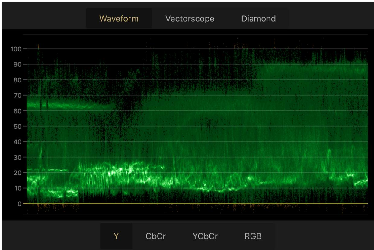
In the waveform scope there are four different displays. Y Displays luminance, CbCr displays color difference, YCbCr combines the first two and RGB shows the red, green, and blue components in the video. The buttons at the bottom of the view makes it easy to select the preferred data.
