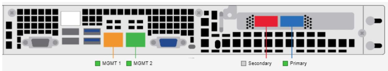
Connect one or both of the management cables. Please note that with the default configuration MGMT 1 (Orange) is configured with a static IP, and MGMT 2 (Green) is configured using DHCP. If you choose to use the static port, the pre-configured address will be 10.0.20.101/24.
