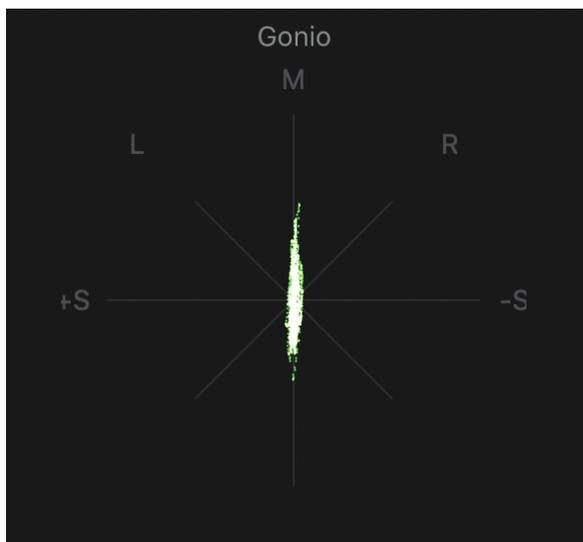
A signal is plotted on each axis. A left-only channel will run a line from top left to the bottom right on the L axis, and a right only channel will make the equivalent line on the R axis. A mono signal will form a straight line in the M axis or be slightly angled according to balance. A stereo signal on the other hand is not symmetrical and will form a jittery cloud. If one of
