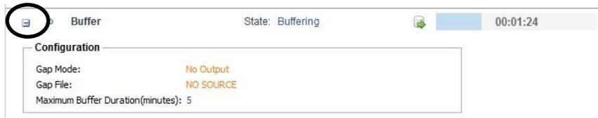
The Configuration window includes information regarding the Gap Mode and Gap File. It further includes the Maximum Buffer Duration listed in minutes. Recall that the Gap Mode permits selection of what you want to be outputting when there is no TS stream available to output from the buffer. A transport stream file may be selected to output during a gap condition by setting the Gap Mode to Default File. A selected file for this is indicated in the Gap File field of the Configuration window.
