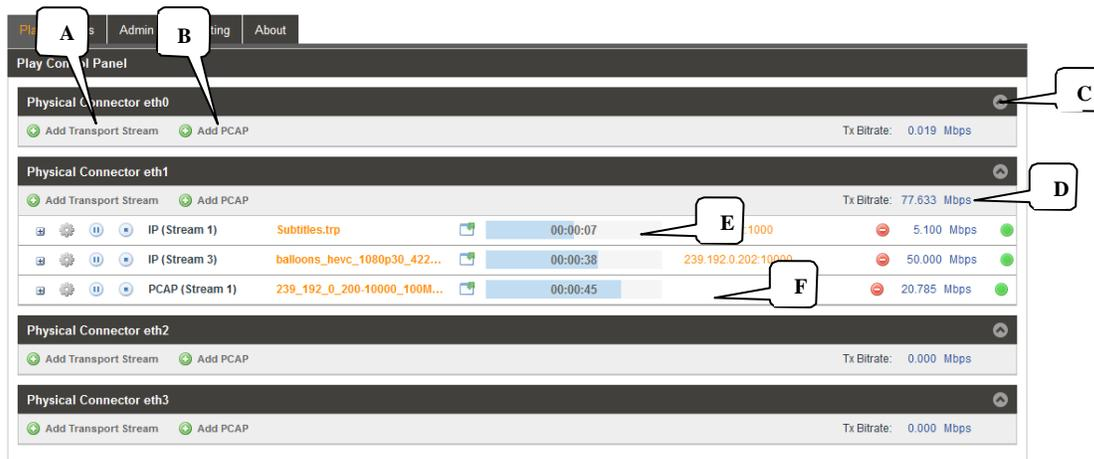
Each Ethernet port section includes some common control fields. The following table provides an overview of the common fields in the Play Control Panel.
