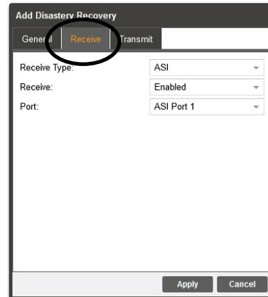
When the Receive Type is ASI, the Receive menu provides selection for enabling or disabling the input port. It further provides selection of one of the available ASI hardware ports. Set the Receive field to “Enabled” to start receiving and buffering the incoming stream. Click on the dropdown in the Receive field and select “Enabled” to make the selected ASI port active.
