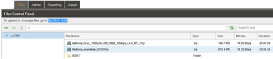
The FTP server address is located in the File Viewing Panel (Files tab) in the TSS 6220's web GUI. Look near the top of the page under the Files Control Panel header. (See circle in illustration) Click at the end of the field and drag the mouse to highlight the ftp address. Copy the address – (Keyboard Ctrl-C key sequence).
