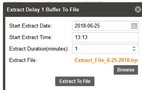
The data extraction requires a duration of time entry in the Extract Duration (minutes) field. Click in the field and enter a value, in minutes. Or click on the up and/or down arrows at the right of the field. The duration must not exceed time stamps currently in the buffer. Reference the time indicated by the Original Time field in the Transmit section and the Delay duration setting to determine applicable start and duration entries for extraction compatibility.
