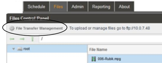
The Configure File Transfer Management menu appears providing entry of enabling/disabling the Username/Password protection. Enabling the Allow Anonymous setting provides anonymous user entry and access. Disabling the Allow Anonymous setting enables the Username/Password user requirement.
