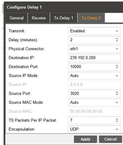
When finished with all the selections in the added TxDelay menu, click on the Apply box at the bottom to apply changes. The delay is added to the Delay Panel. You can access the configuration menus for changes by clicking on the cog wheel
