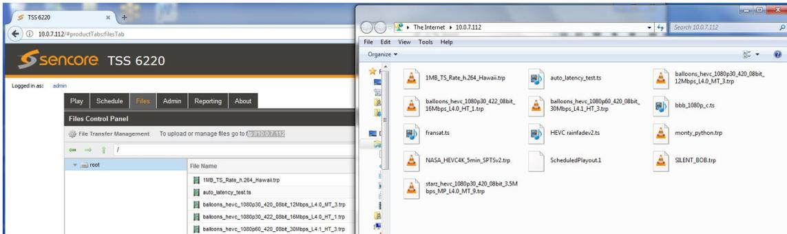
The FTP server address is located in the File Viewing Panel (Files tab) in the TSS 6220's web GUI. Look near the top of the page under the Files Control Panel header. (See circle in illustration) Click at the end of the field and drag the mouse to highlight the ftp address. Copy the address – (Keyboard Ctrl-C key sequence). When using SMB (Samba), copy only the IP address.
