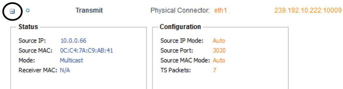
The Status part of the window provides information regarding the Disaster Recovery output status. It includes an indication of its source IP address and its MAC address. It indicates if the output is in a unicast or multicast configuration status. It indicates a MAC address from a destination receiver if applicable.
