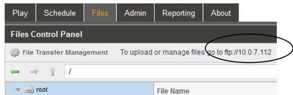
Open a Windows Explorer or File Explorer application window on your PC. In the header of this application – paste in the ftp address listed in the TSS 6220's File menu on the second line below the Files Control Panel heading. Paste the ftp address – (Ctrl V). For SMB protocol, enter backslash key entries and paste only the IP address listed into the Control Panel address line of Windows Explorer. See example below.
