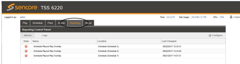
The **Reporting** tab in the TSS 6220 contains logs for active alarms currently affecting the unit and an event log. The active alarms are updated periodically in order to reflect the real-time state of the unit. Once an error is cleared it will be cleared from the active alarms window. The event log can be used to view alarm and event history. Both the active alarm and event logs can be configured to hide or change the behavior of alarms and events.
