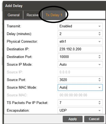
The Tx Delay tab includes settings to define the TSS 6220 as a specific source device for IGMPv3. This allows each steam to be seen by the network as a unique source device with a unique IP address, and/or source port, and/or MAC address. This section provides descriptions of the settings.
