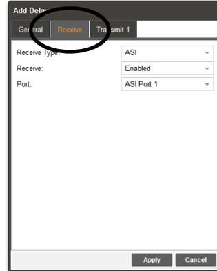
When the Receive Type is ASI, the Receive menu provides selection for enabling or disabling the input port. It further provides selection of one of the available ASI hardware ports. Set the Receive field to “Enabled” to start receiving and buffering the incoming stream. If the Receive field is set to “Disabled” the incoming TS stream on the selected port is not received or routed to the delay buffer.
