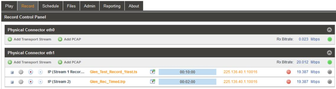
The record feature provides manual recording in which a user may control the start and ending of the record segment. A user may also perform a scheduled record event in which the duration of the timed recording may be specified along with the start date and time.
