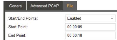
When starting and ending points are specified and enabled, the playback windows observed in the Playback Control Panel change to indicate the start/end limits that are specified. Brackets indicate the starting and ending points.
