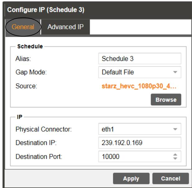
Define the IP parameters in the IP section. Verify that the Physical Connector field indicates the desired Ethernet port. If not, select the Ethernet port you wish to output the stream. Enter the Destination IP and the Destination Port values. Click on the Destination IP field and enter the destination address. Click on the Destination Port field and enter a Destination Port. Click on the Apply box to add the schedule to the Schedule Control Panel under the respective Ethernet port.
