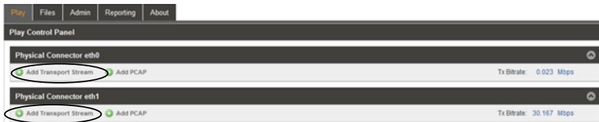
The Play Control Panel is simplified for viewing with a Hide/Show streams feature for each Physical Connector eth section. To show all the streams outputting to an Ethernet port click on the Show/Hide icon
