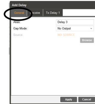
The Gap Mode importantly defines what the output is when there is no output transport stream to output from the delay buffer. This occurs when the buffer is buffering and has not yet reached the specified delay time. It also occurs when the input TS stream is lost and the buffer streams out until it is depleted. It can also occur when bad data is contained in the buffer because of an input stream issue.
