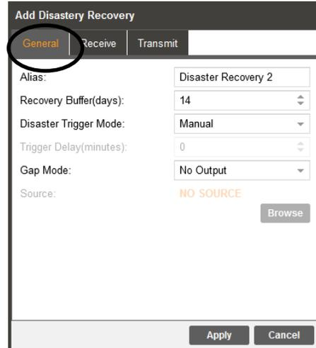
The Gap Mode importantly defines what the output is when there is no output transport stream to output from the delay buffer. This occurs when the buffer is buffering and has not yet reached the
