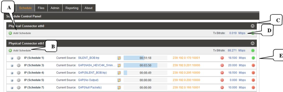
Each Ethernet port section includes some common control fields. The following is a general overview of items in the Schedule Control Panel and description of some common fields. The remainder of this chapter describes definition of the fields and configuration menus.
