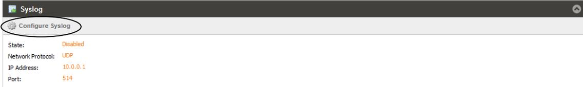
To configure the Syslog, click on the Configure Syslog icon
