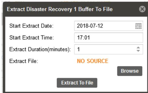
The data extraction requires a defined duration which is determined by an entry in the Extract Duration (minutes) field. Click in the field and enter a value, in minutes. Or click on the up and/or down arrows at the right of the field. The duration must not exceed time stamps currently in the buffer. Reference the time indicated by the Original Time field in the Transmit section and the Delay duration setting to determine applicable start and duration entries for extraction compatibility.
