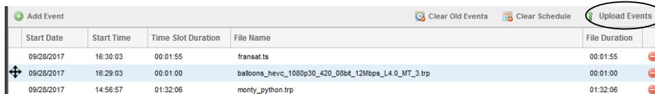
When uploading events, the values in the CSV format must match the columns in the TSS 6220 schedule for date, time, duration, and file naming. File naming must accurately match file naming of play files. Below is a sample file showing CSV formatting.
