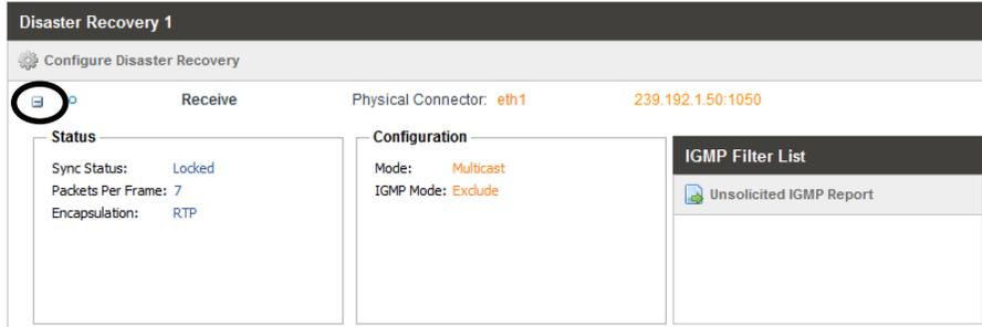
The Sync Status, Packets Per Frame and Encapsulation fields provide information regarding the incoming receive transport stream. Should the Sync Status indicate “Unlocked” check the IP configuration settings and/or availability of the MPEG-IP stream.
