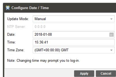
Enter the NTP Server address in the address field. Click the Apply field.
