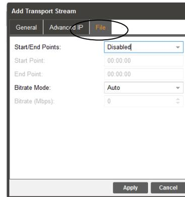
The Bitrate Mode provides an automatic setting in which the TSS 6220 automatically determines the ideal playout stream rate. You can set the Bitrate mode to Manual when you wish to increase the output bitrate. In the manual mode, click on the up and/or down arrows in the bitrate field to increase or decrease the bitrate in Mbps.
