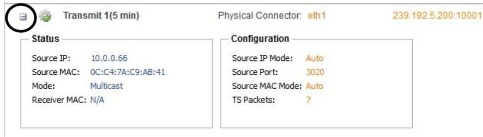
The Status part of the window provides information regarding the Delay’s output status. It includes an indication of its source IP address and its MAC address. It indicates if the output is in a unicast or multicast configuration status. It indicates a MAC address from a destination receiver if applicable.
