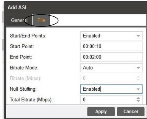
You can enter starting and ending times within the play duration time of the ASI play file. You can enable or disable the playout to conform to these entered start point and end point times. Set the Start/End Point field to “Enabled” and enter the Start Point and End Point.
