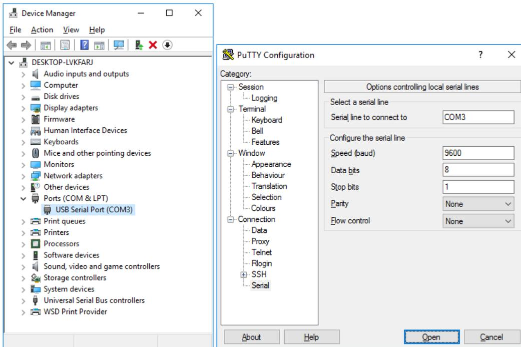
Figure 4.13: Connecting to the serial console over USB
