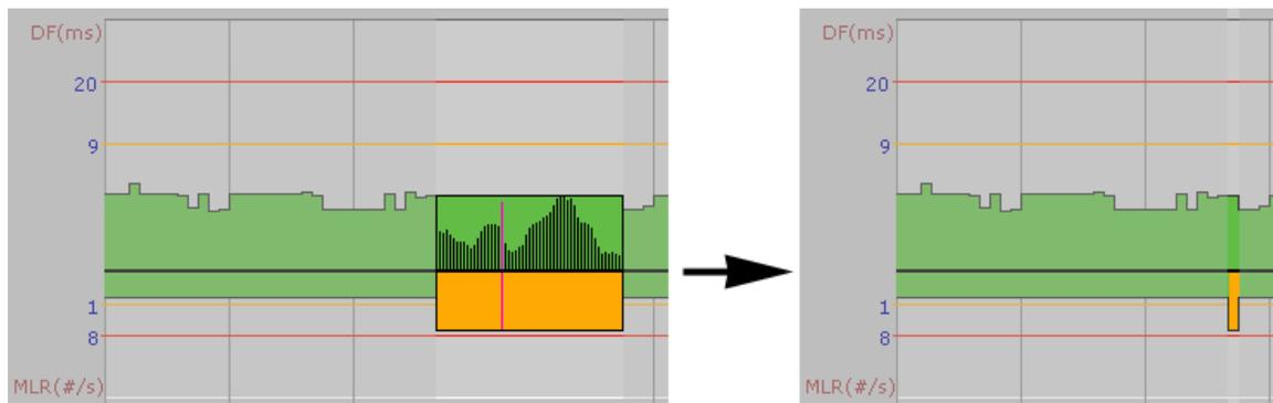
*The pink line indicates a packet loss of 6 or 7 and a doubling of the jitter component.*
