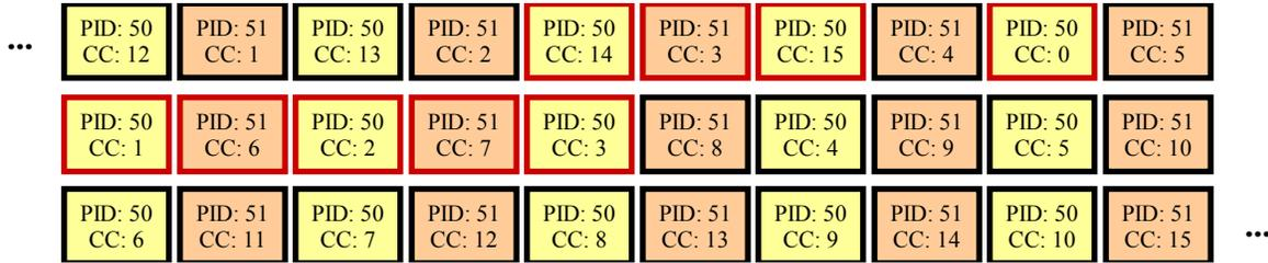
When the Transport Stream reaches our imaginary head-end some packets (those with red frame) have been lost (maybe due to a bad satellite connection). Our IP-Streamer packs 7 and 7 MPEG-2 TS packets into each UDP-frame (mapping is 7TS/UDP) and the resulting frames may look like:
