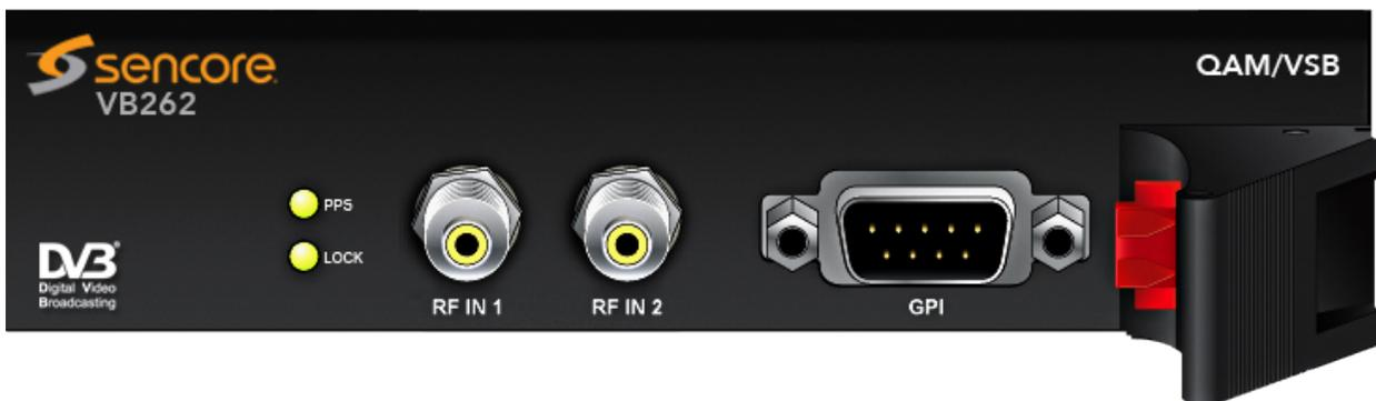
The VB262 QAM/8VSB demodulator is an optional input interface module. It has two RF inputs; one or two of these are enabled according to probe licensing.
