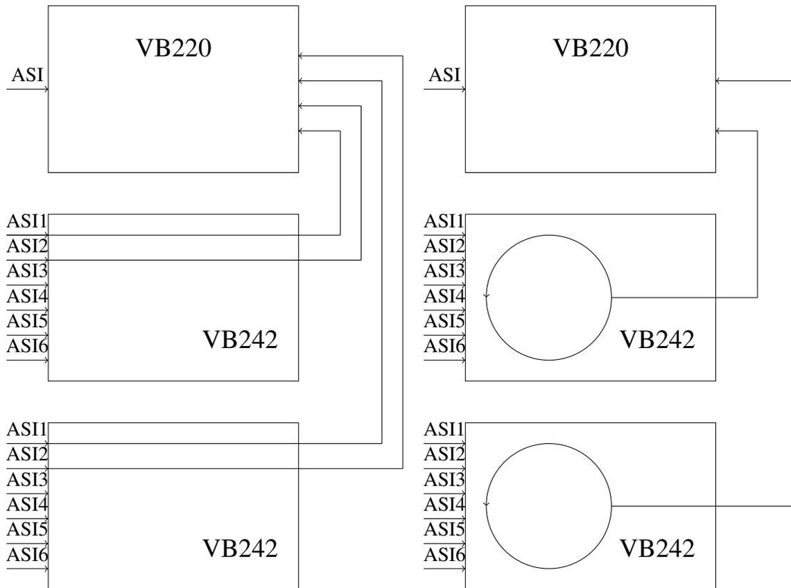
The figure above illustrates signal routing for two VB242 modules in one chassis, for continuous monitoring mode and round-robin mode respectively. The circles represent round-robin functionality, where the ASI inputs can be monitored sequentially. In continuous mode five ASI signals may be analyzed in parallel by the probe module, whereas in round-robin mode three ASI signals are analyzed in parallel.
