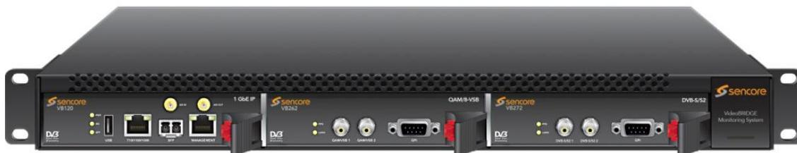
Figure 4.1: The Enhanced Chassis with probe boards installed
