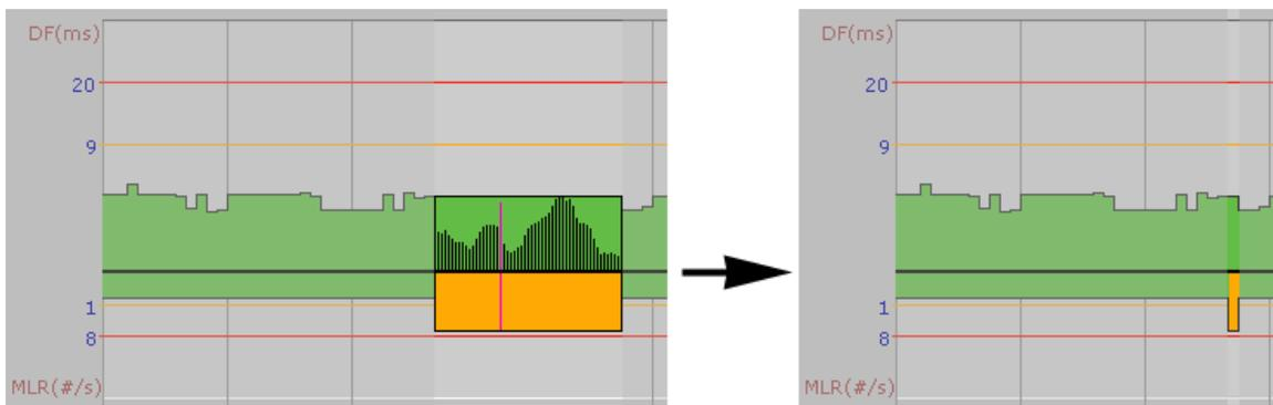
*For VBR streams a similar packet-loss will not necessarily affect the IAT graph even if the time between two neighboring packets doubles. The pink line represents the IAT and MLR value measured for the missing packet.*
