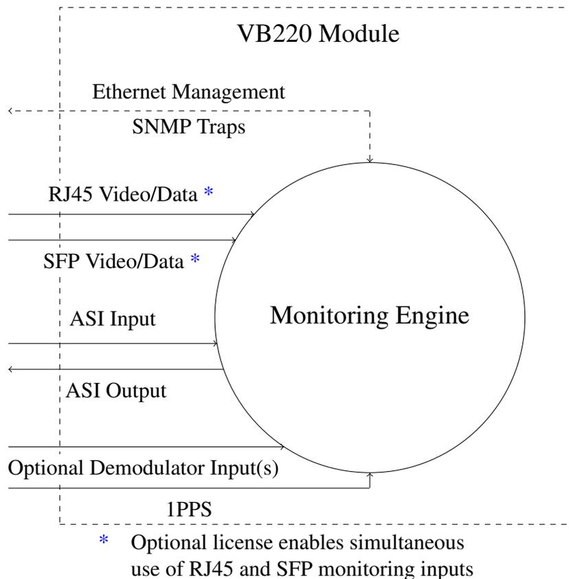
Figure 2.1: The VB220 Module – Principle of Operation
