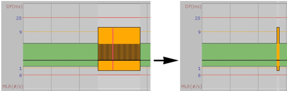
*If a UDP packet goes missing after it has left the router it will visually affect both the IAT and MLR for CBR streams. The pink line represents one elementary measurement.*
