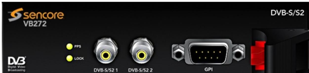
The VB272 DVB-S/S2 Demodulator is an optional input interface module capable of receiving DVB-S (QPSK) and DVB-S2 (8PSK, 16APSK, 32APSK) signals. The module has two RF inputs. The second input can be activated through a software option key.
