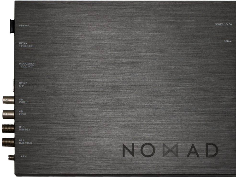
Figure 4.1: The NOMAD portable probe
